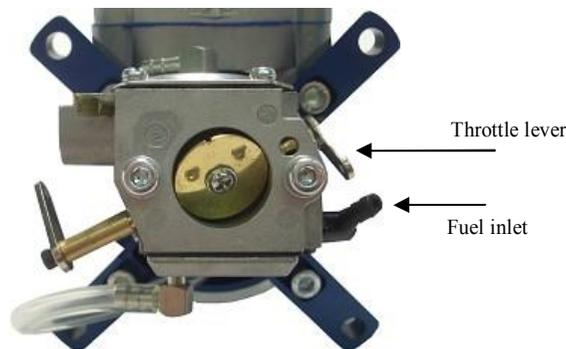
Caution! Never tighten the adjusting needles with too much strength. This may cause damage of the needles. If the needles are damaged this way it is no longer possible to adjust the carburetor and it is necessary to exchange it for a new one.
