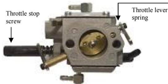
If the throttle pull rod is not equipped with flexible element it is recommended NOT to put off the throttle valve spring. Otherwise the vibrations of the engine can cause excessive wear of the throttle valve shafting and with this deteriorate the carburetor function.
